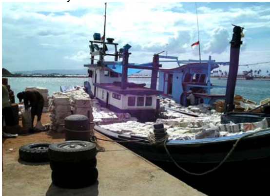
Packed bricks loaded manually to wooden coaster
