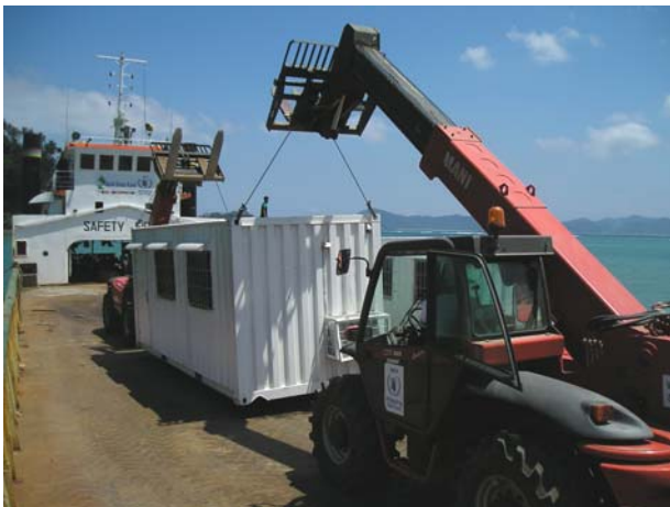
Two Forklifts Manitou working together to discharge the container at Pulo Aceh
